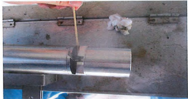
Checked or Cleaned Optical module (Lamp , lens)
